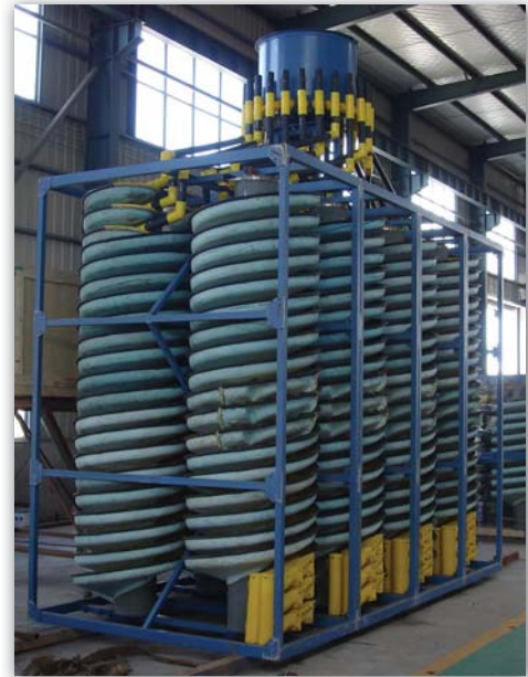
The Krebs CPX spiral can be retro-fitted into an existing 5-turn spiral frame giving enhanced performance equivalent to that of a conventional two stage spiral installation.
